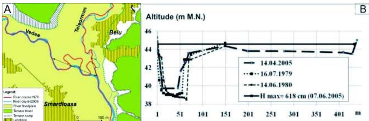
Fig. 4. The Vedea riverbed dynamics at Teleorman junction (in plans - A and cross section - B) (downstream Alexandria weather station) (after A.N.A.R. – D.A.A.V, 2008, with modifications)
